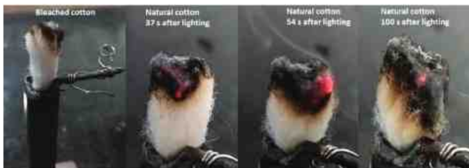
Figure 11. Pictures of smouldering of cotton strand, d = 25 \text{ mm} , \rho_f = 70 \text{ kg/m}^3 at different times.
