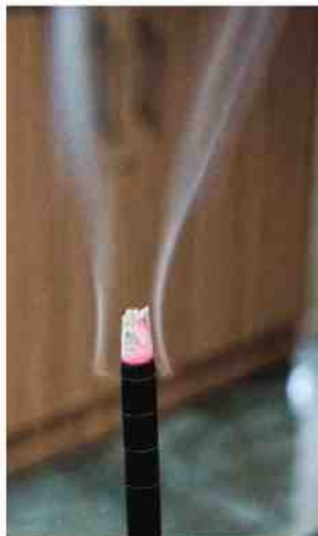
Figure 1. Photograph of a smoldering incense stick with volatiles issuing from all around below the red hot zone.
