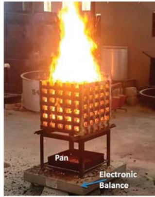
Figure 3. Experimental arrangement used in the dry chemical powder qualification tests and crib during its peak burn rate.
