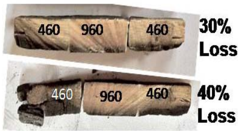
Fig. 2 a Coupled density wood samples (numbers are in kg/m^3 )
