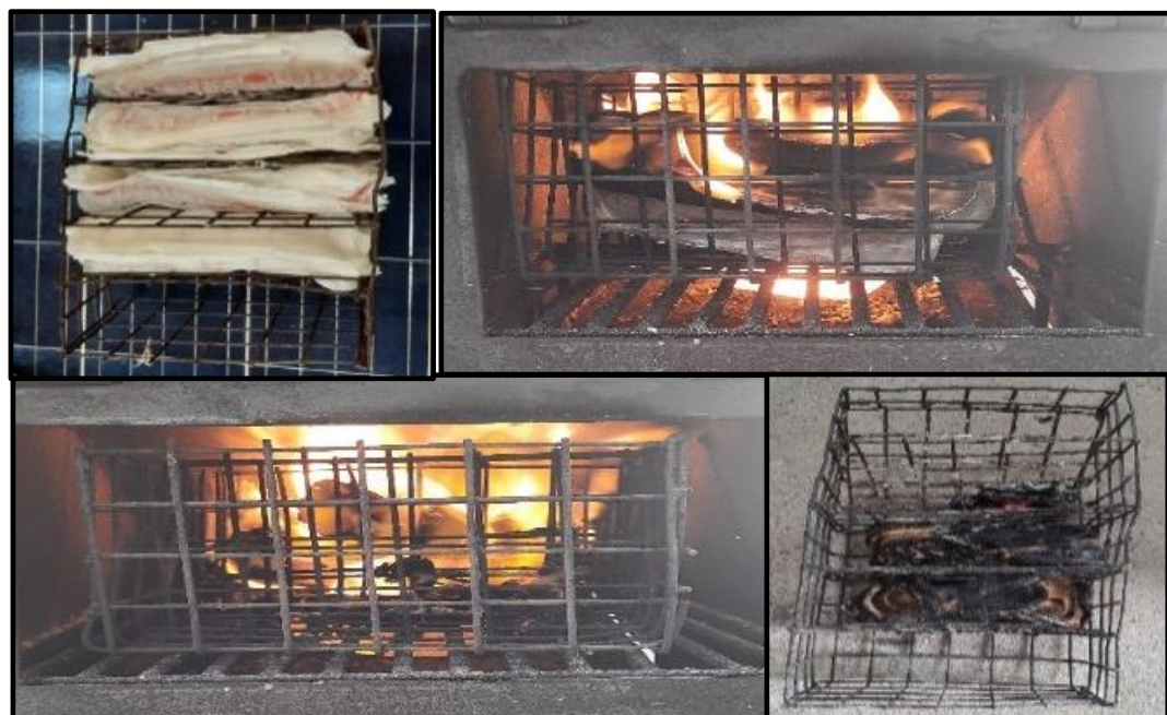
Figure 4 Burning of sanitary pads loaded on to the tray
