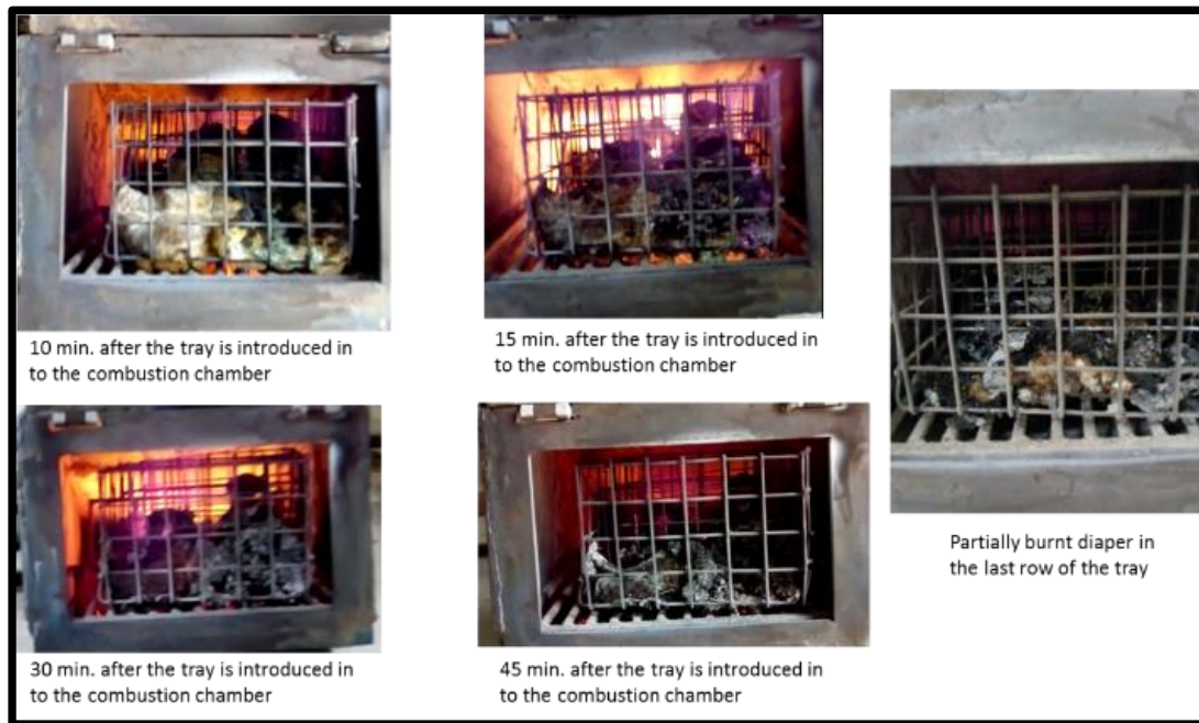
Figure 5 Burning of diapers loaded on to the tray
