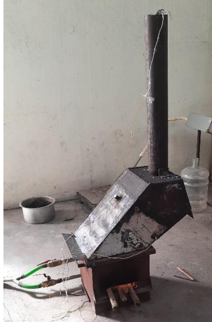
Figure 3 Sanitary pad/diaper disposal system Prototype
