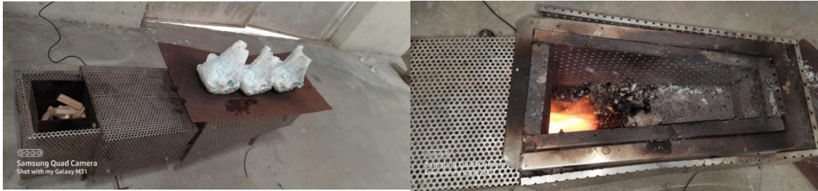
Figure 2 a) Wet Diapers kept on the stove b) Diapers shown directly on the flame
