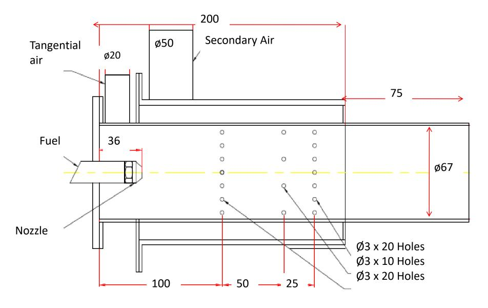
SS combustion chamber is 70 mm internal diameter with tangential air supply at the head end and through two rows of 2 mm dia holes, ten in each row on the periphery of the inner shell.
