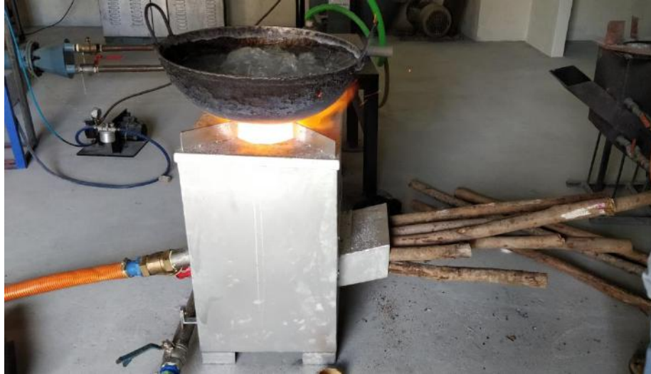
A 15 kg/hr VEBCOD system in operation (Synergy pvt ltd)
