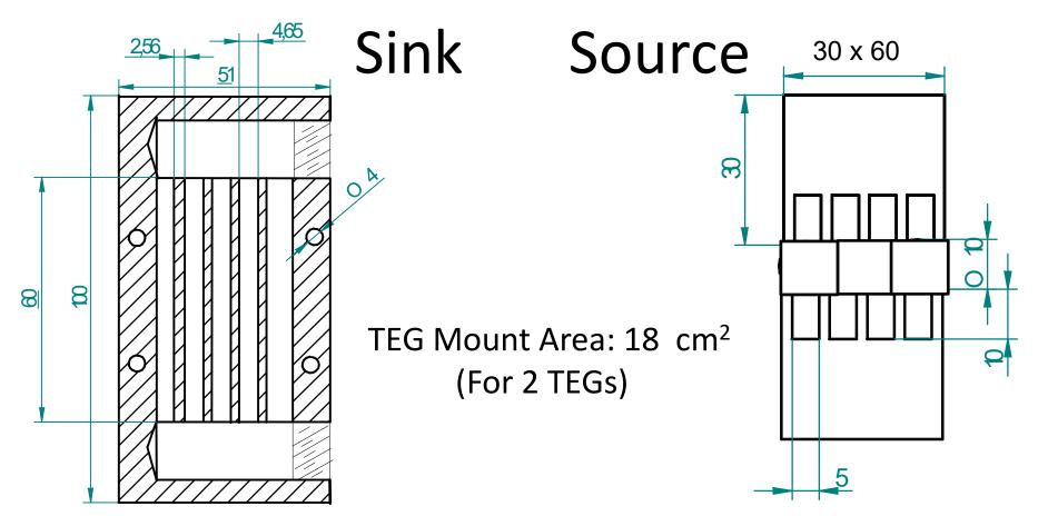
Al body, Water Flow: 1 *l*/min TEG heat flux = 13 W/cm<sup>2</sup> Water Vel. = 0.2 m/s HE area = 44 cm<sup>2</sup> Heat Flux to water = 5.4 W/cm<sup>2</sup> Al Body, Hot Face T: 300 <sup>o</sup> C Fin base T: 311<sup>o</sup> C, Gas Avg. T: 750 <sup>o</sup> C HT Coeff: 9 W/m<sup>2</sup>K Fin surface Heat Flux: 3.8 W/cm<sup>2</sup>
