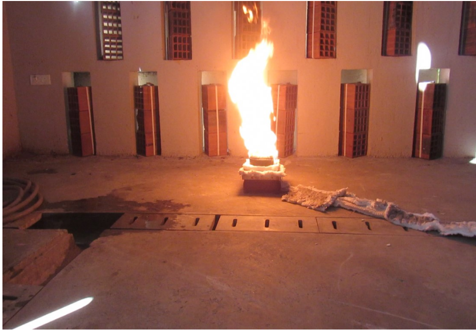
Diffusion flame without external air supply
