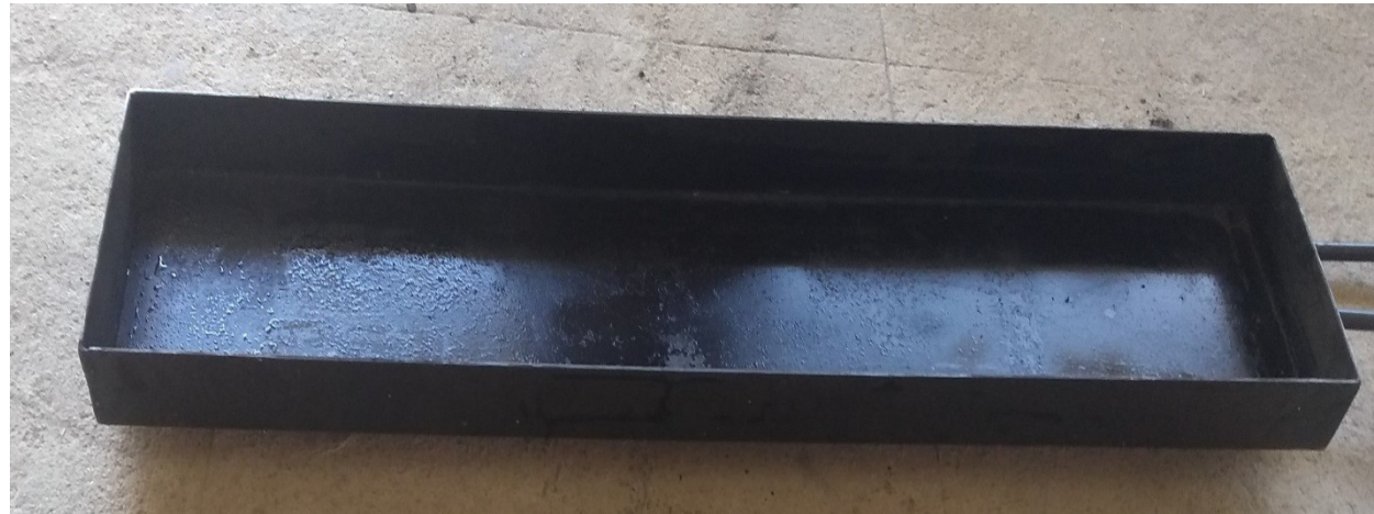
1 m long x 0.2 m wide x 0.06 m high rectangular, MS Pan
